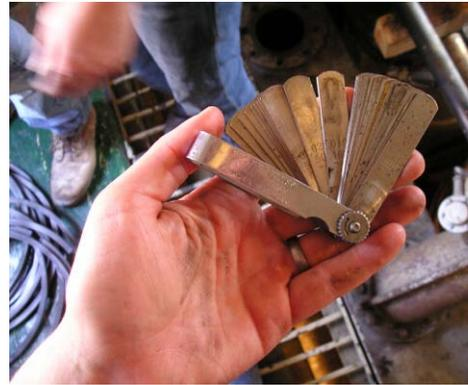
Feeler gauges, used to take precise measurements
