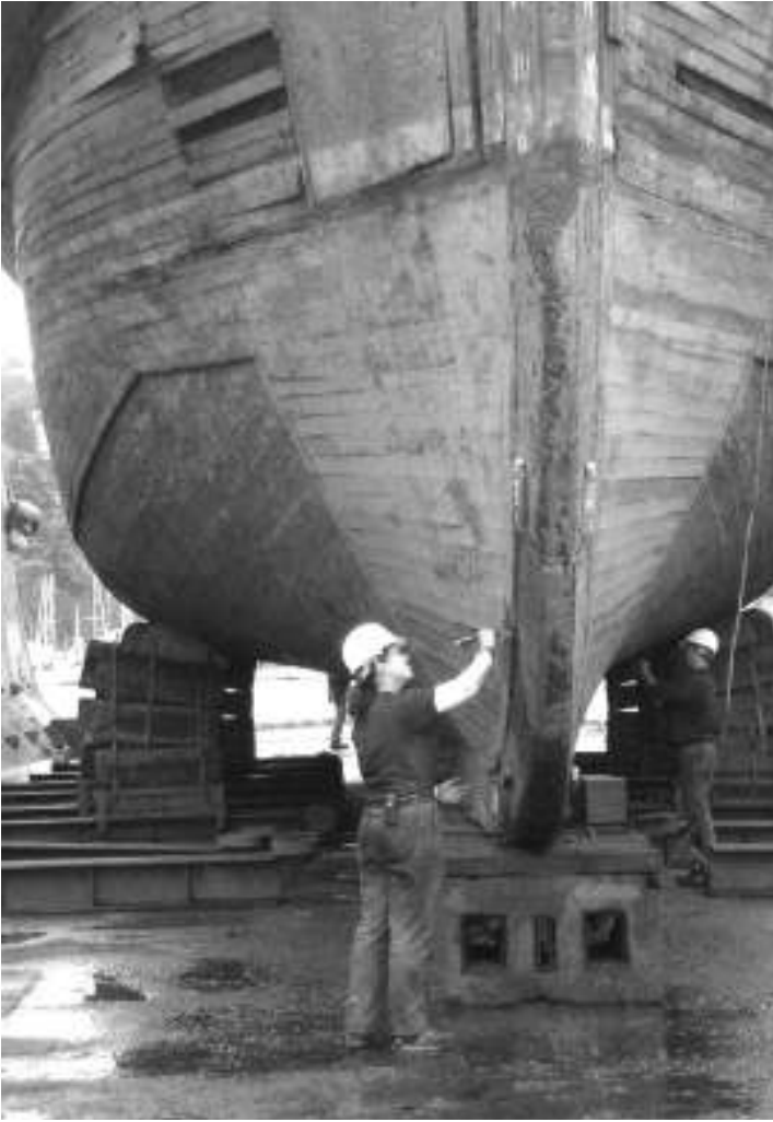
The Arthur Foss 's bow during the 2007 haul-out. The ironbark sheathing shows from the turn of the bilge to the rubstrakes.
